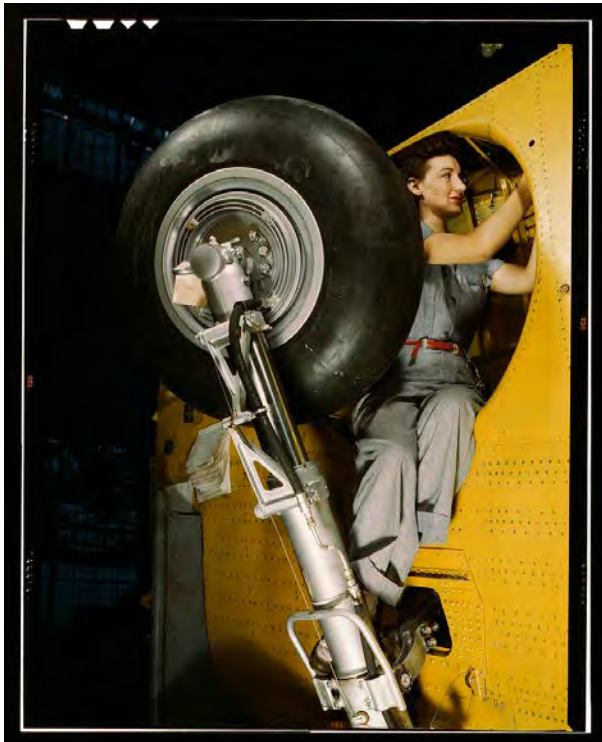
This woman worker at the Vultee-Nashville is shown making final adjustments in the wheel well of an inner wing before the installation of the landing gear, Nashville, Tenn. This [is] one of the numerous assembly operations in connection with the mass production of Vultee "Vengeance" dive bombers [Feb. 1943]
