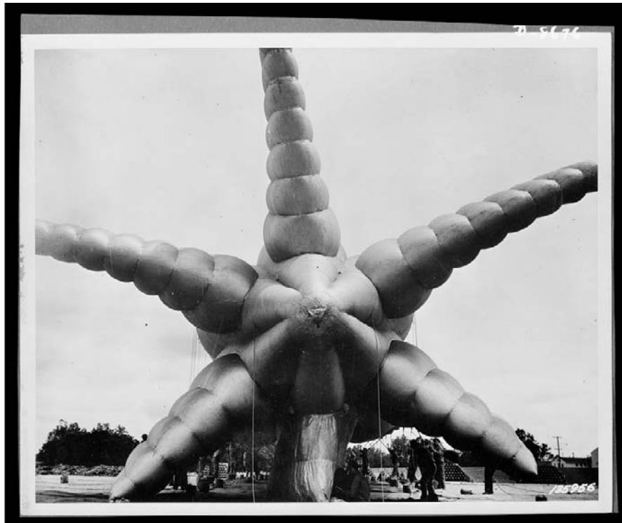
Balloon barrage training center. Aerial octopus. This strange looking creature is a tail view of one of the barrage balloons prompting the above title. The lower fin is filled with gas last as it is slowly raised from the ground. Camp Tyson, Tennessee [1940-1946]
